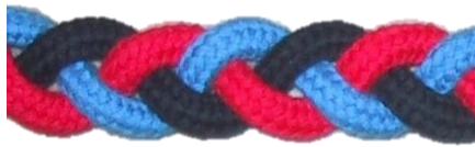
Braiding creates a composite “rope” that is thicker and stronger than non-interwoven fibers.
